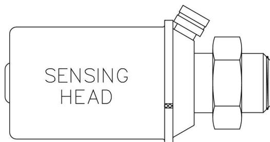
The sensing heads are attached to the process line by Isolation Valves. These adapters must not be placed in an area where vibration is severe or excessive. They should be installed a minimum of six feet apart to prevent interaction of the purges.
