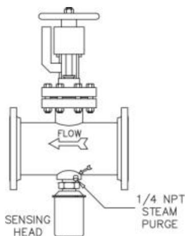
If the sensing head is to be mounted on a vertical pipe, the fluid flow should be upward. The arrow on the adapter should point in the direction of fluid flow. (See Sensing Head to Adapter Positioning.) The probe end of the sensing head has a groove for an interface o-ring.
