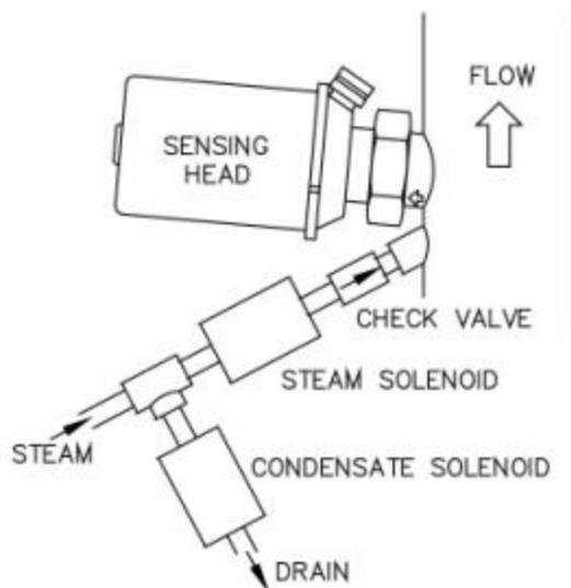
Steam pressure must be at least 50 psi (3.44 bar) above process pressure but less than 100 psi (6.89 bar) above process pressure with adequate condensation drainage at the steam valve in order to ensure hot steam for cleaning the prism. Trial and error must, of necessity, be employed in determining the minimum steam time necessary for proper steam cleaning of the prism due to variables from application to application.
